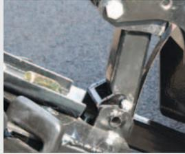
To raise the plow, lift plow by handle to the manual latch rung lock and then lower. This will lock the plow in the raised position. Then add safety pin.
