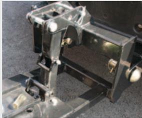
To lower the plow, lift the plow by the handle up past the manual latch rung lock and then lower to the ground. The manual latch rung lock works just like an extension ladder.
